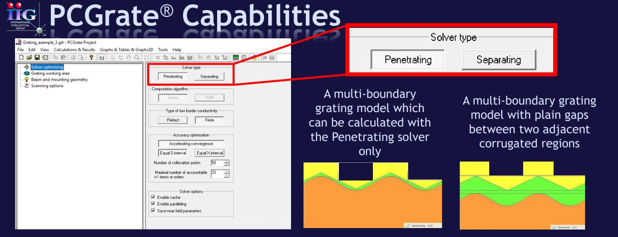
There are two types of solvers available in **PCGrate**®, i.e. *Penetrating* and *Separating*. The solvers have different behavior and mutually complementary capabilities for many difficult cases such as coated gratings with thin layers, randomly rough periodical or non-periodical structures, grazing incidence, and photonic crystals.
